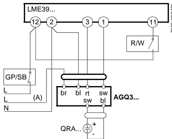
Measuring circuit for measuring the UV detector current
