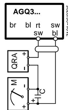
Measurement made at the UV detector QRA...
